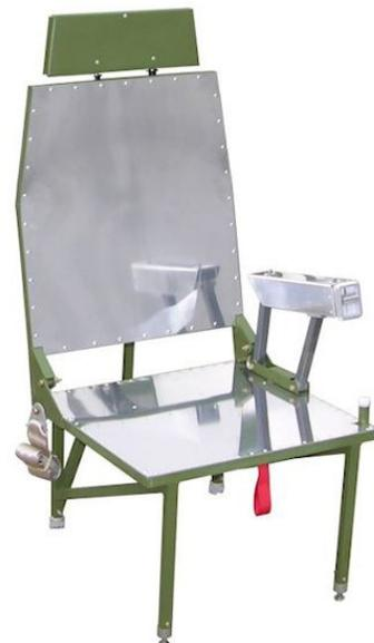
**Description:** AvFab's King Air Econo Seat is our sleek, airline style, high density commuter seat that allows for up to 9 passengers in a King Air 200 and 11 passengers in a B300. The seats are extremely robust and are being used world-wide in the most demanding conditions and environments. Weighing only 22lbs, their strength to weight ratio is unmatched. No requests for spare parts or repairs have been made. Delivered in "green" ready to be finished condition. Upholstery is available.
