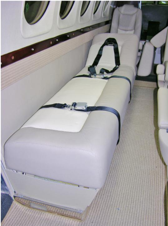
The stretcher/divan quickly and easily converts between passenger and patient configurations. You can carry passengers on one leg of a flight and then convert it for an ambulatory person on the next leg. Occupancy in either configuration is FAA-approved during all phases of operation.
