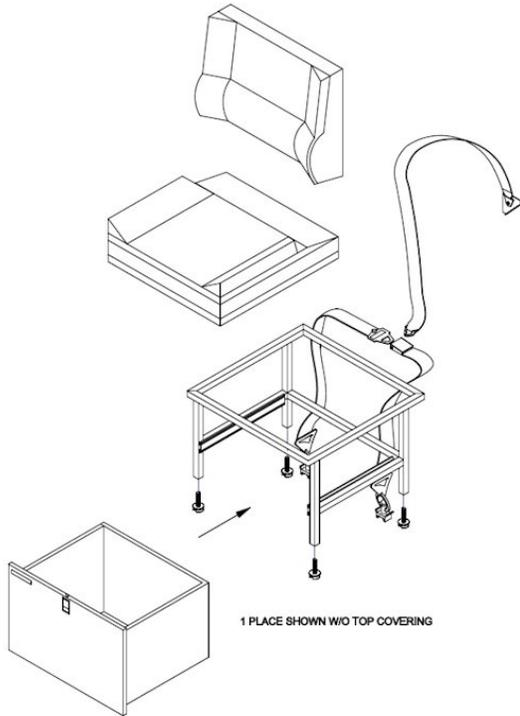
Line Drawing shows how the seat belt harness is attached.
